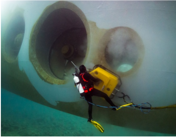
Figure 2: Conditioning/cleaning of the main hull of a large cruise ship.
