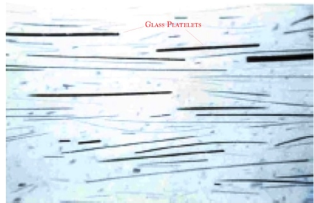
Figure 1: Microscopic cross-section view of a commercially available STC formulated as a vinyl ester with embedded glass flakes.
