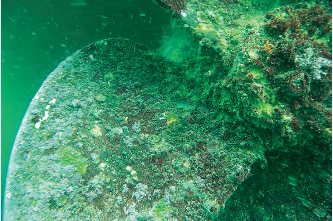
Very badly fouled propeller.
