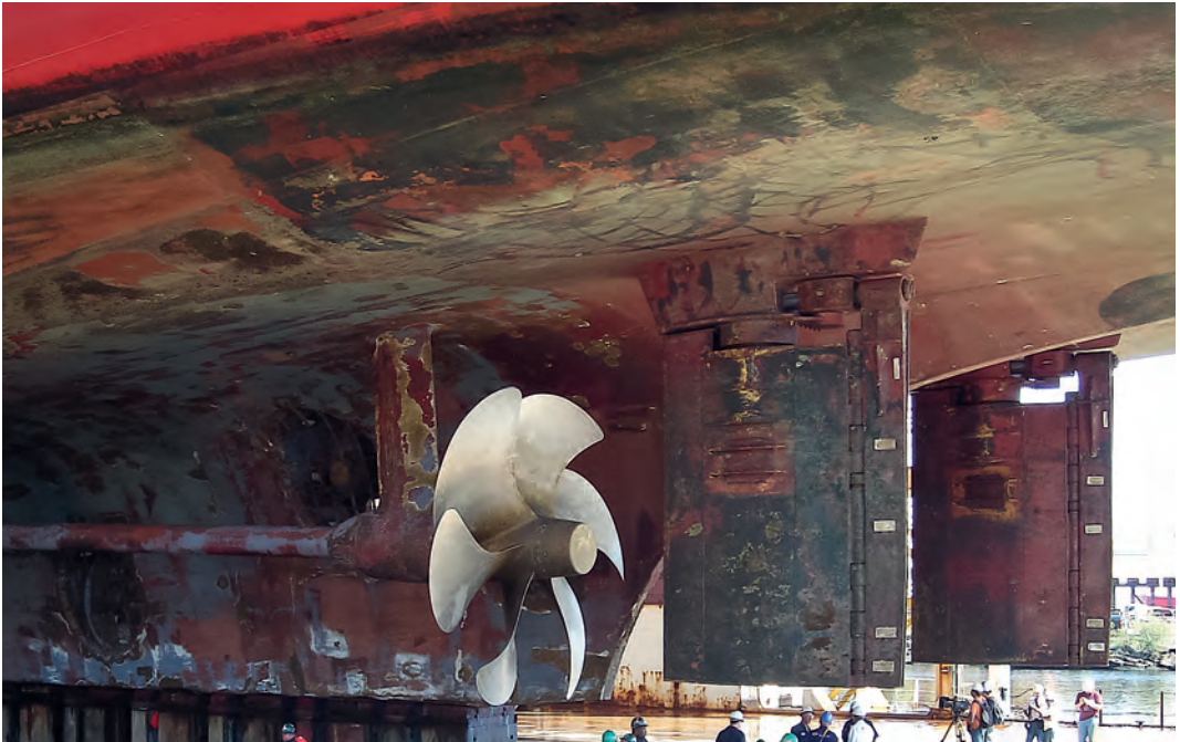
Ship in dry-dock showing typical antifouling paint condition after fouling removed.
