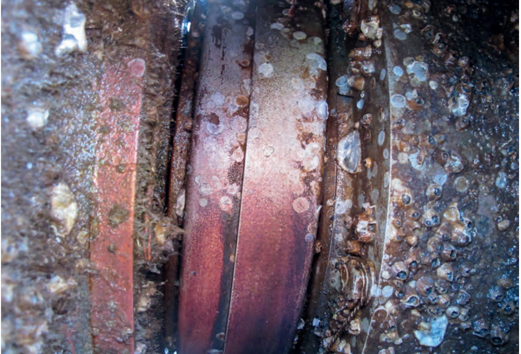
Macrofouling around the propeller shaft area of a hull coated with biocidal antifouling.
