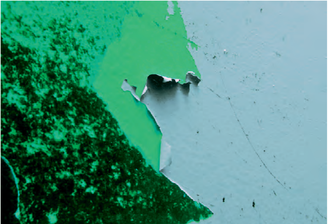
A partially cleaned silicone fouling release showing damage and fouling.
